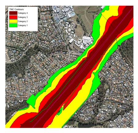
Figure 6: QDC noise contours for the first floor
