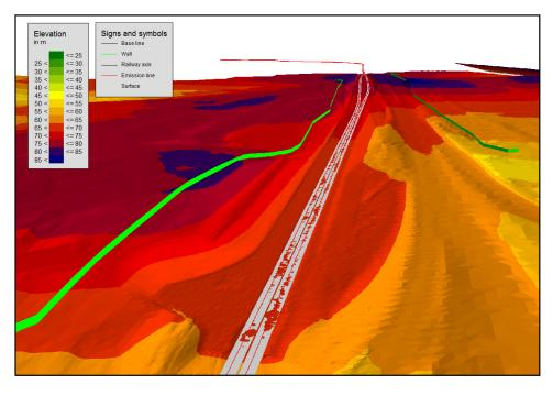
Figure 3: Terrain model snapshot with noise barriers
