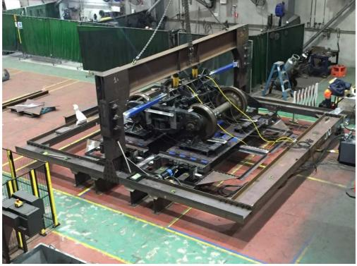
Figure 3 the Transport for NSW bogie warp stiffness test rig
