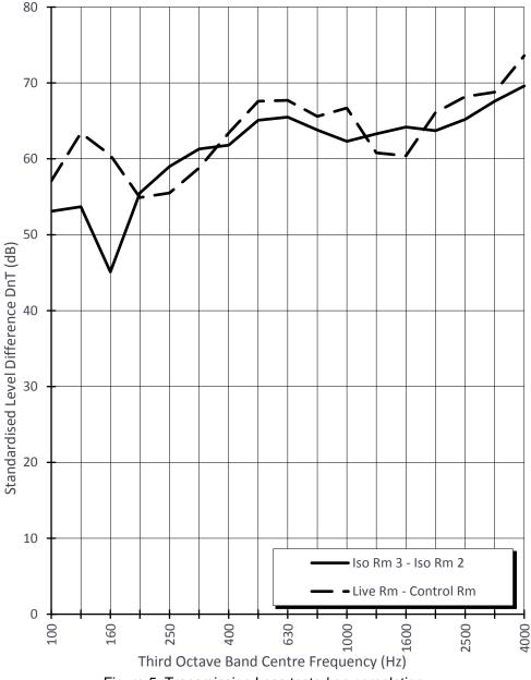
Figure 5: Transmission Loss tested on completion
