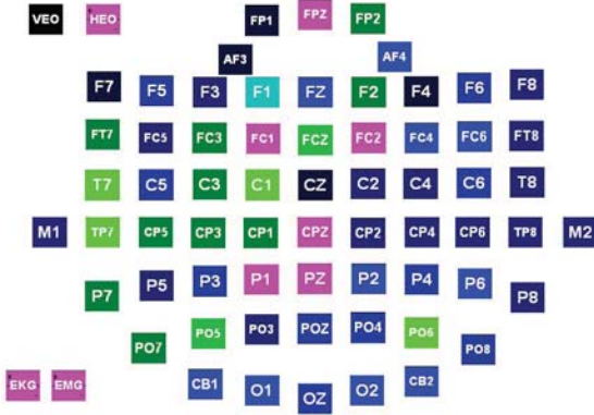
Fig. 4. EEG cap channels location (different colours indicate different impedances on the corresponding electrodes with blue good impedance and pink bad impedance)
