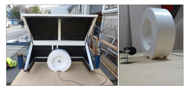
Figure 3. Artificial sound source inside and outside a CPX trailer (University of Canterbury)
