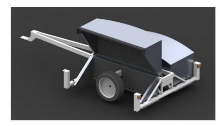
Figure 2. Visualisation of the University of Canterbury CPX trailer (University of Canterbury)
