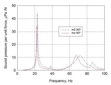
Figure 9. Spectra of sound pressure radiated by cylindrical shell at range 1000 m on a colatitude of  $90^{\circ}$ , for the m0 and ms cases. Longitude mode n = 0.
