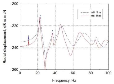
Figure 8. Spectra of radial displacement for the n = 0 longitude mode at x = 9.27 m, obtained for the m0 (not stiffened) and ms (stiffened) cases.
