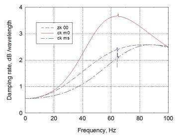
Figure 3. Spectra of axial damping coefficient for the three cases examined. The symbols in the legend have the same meaning as in Figure 2.
