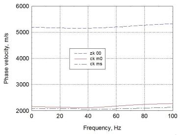
Figure 2. Spectra of axial phase velocity for the three cases examined. In the legend, 'zk 00' denotes the [1] case which had no added mass or stiffening, 'ck m0' denotes the [2] case with no stiffening, and 'ck ms' denotes the [2] case with stiffening.
