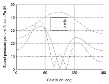
Figure 10. Magnitude of sound pressure radiated by cylindrical shell at range 1000 m as a function of colatitude, at the shell's first three harmonic frequencies for the m0 case (23 Hz, 47 Hz and 72 Hz). Longitude mode n = 0.
