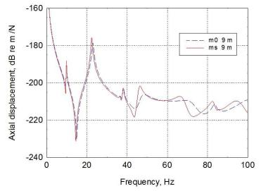
Figure 7. Spectra of axial displacement for the n = 0 longitude mode at x = 9.27 m, obtained for the m0 (not stiffened) and ms (stiffened) cases.
