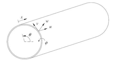
Figure 1. Coordinates and displacements (u,v,w) for a thin cylindrical shell. The radial coordinate is not depicted. The angle  $\phi$  denotes the (small) slope of the shell wall in the (negative) axial direction.
