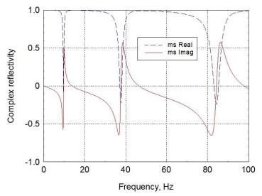
Figure 6. Complex reflectivity of shell axial displacement waves incident at a shell end, for the ms case from [2].
