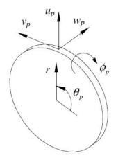
Figure 4. Polar coordinates and displacements for a thin end plate. The axial displacement  $w_p$  is transverse (perpendicular) to the plate. The angle  $\phi_p$  denotes the (small) slope of the plate in the axial direction.
