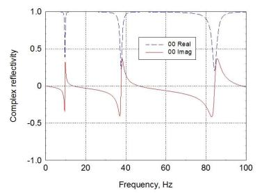
Figure 5. Complex reflectivity of shell axial displacement waves incident at a shell end, for the ZK00 case from [1].
