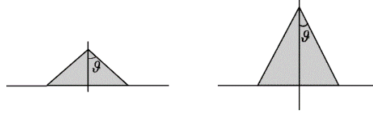
Figure 1. (a) Edge half-angle \vartheta greater than 45^\circ to the mean flow direction and (b) Edge half-angle \vartheta less than 45^\circ to the mean flow direction.
