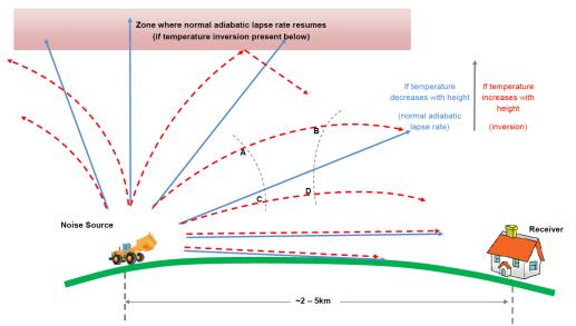
Figure 2. Influence of temperature inversions on propagation of noise
