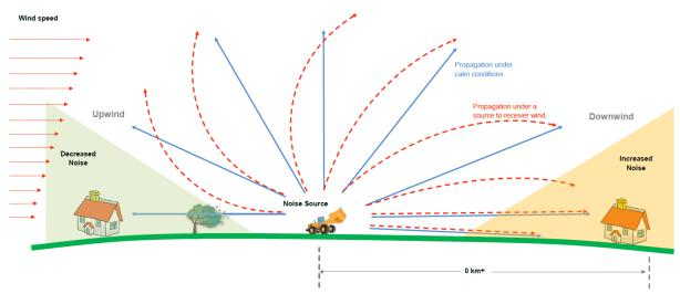
Figure 1. Influence of wind on propagation of noise
