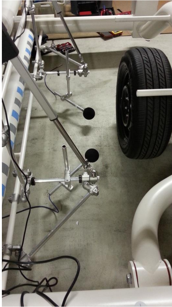
Figure 2. Microphone frame support structure for left tyre viewed from front of trailer
