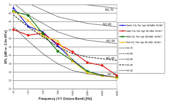
Source (Allen, 2015) Figure 4: Acoustic levels measured on-orbit in ISS US Crew Quarters with fans on high-flow setting.
