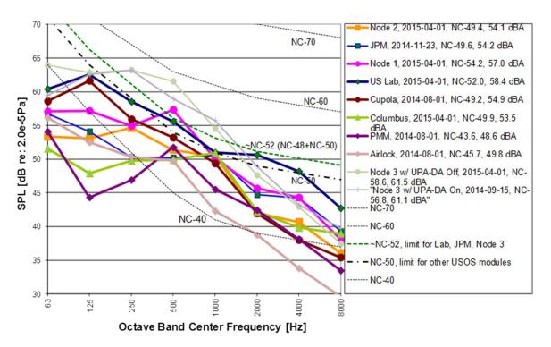
Source (Allen, 2015) Figure 3: Acoustic levels measured on-orbit in ISS US Segment Modules.
