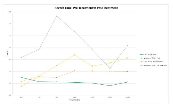
The graph above summaries the EASE modelling before and after treatment and also the measured reverberation time before and after treatment. The EASE modelling showed large flutter echoes and standing waves which were not picked up by the measured data. However, with 45 *Whisper* panels, there was a significant difference in the modelling data and also the measured data.
