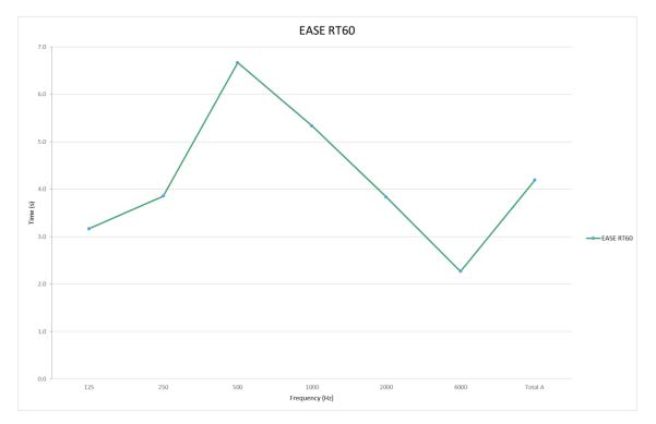
The modelled reverberation time in EASE calculated an overall RT of 4.2 seconds. Graph below shows the comparison with measured and modelled data.
