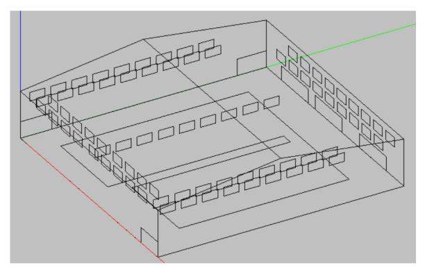
Floorplan (RSA, 2017) Figure 4: Hanging Baffle EASE modelling
