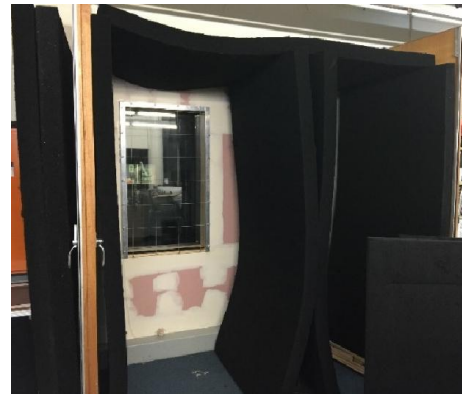
Figure 3 - 'Absorptive Tent' in receiver room, with the rear sheets of absorptive material (those closest to the camera) removed.
