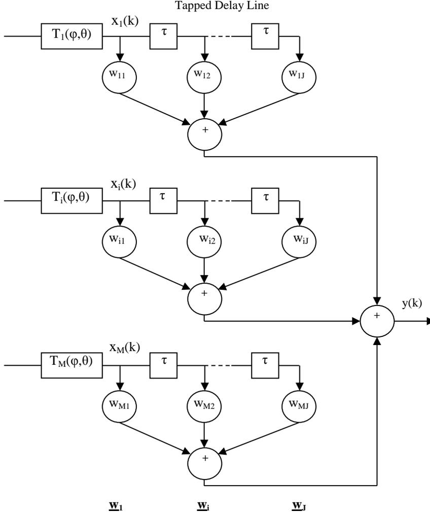
Figure 1. Adaptive beamformer structure using TDL filter
