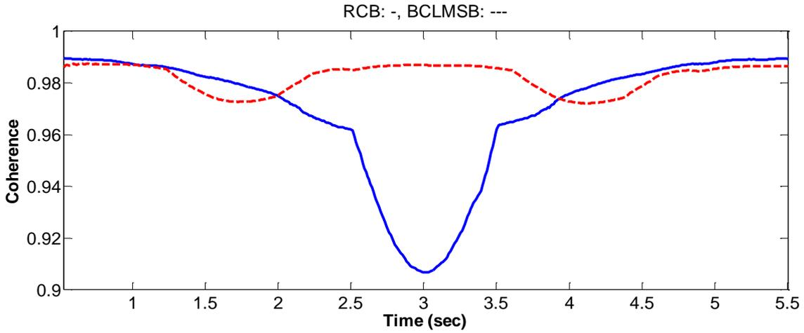
Figure 3. Time history of coherence of RCB and BCLMSB, with the signal source moving from  $-1.2^\circ$  to  $1.2^\circ$  at a bearing rate of 0.4 degree/second. The time averaged coherences of RCB and BCLMSB are 0.9703 and 0.9825, respectively.
