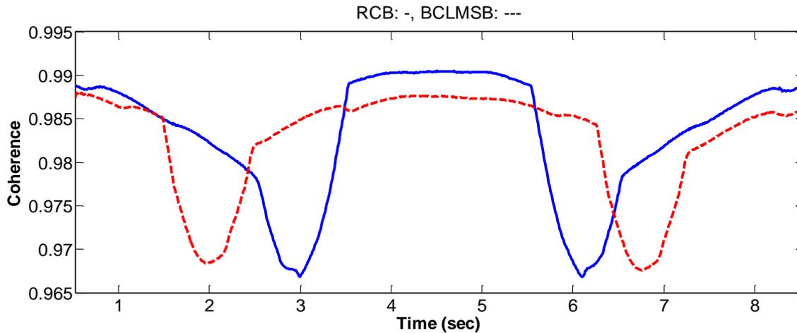
Figure 2. Time history of coherence of RCB and BCLMSB, with the signal source moving from  $-0.9^\circ$  to  $0.9^\circ$  at a bearing rate of 0.2 degree/second. The time averaged coherences of RCB and BCLMSB are 0.9832 and 0.9831, respectively.
