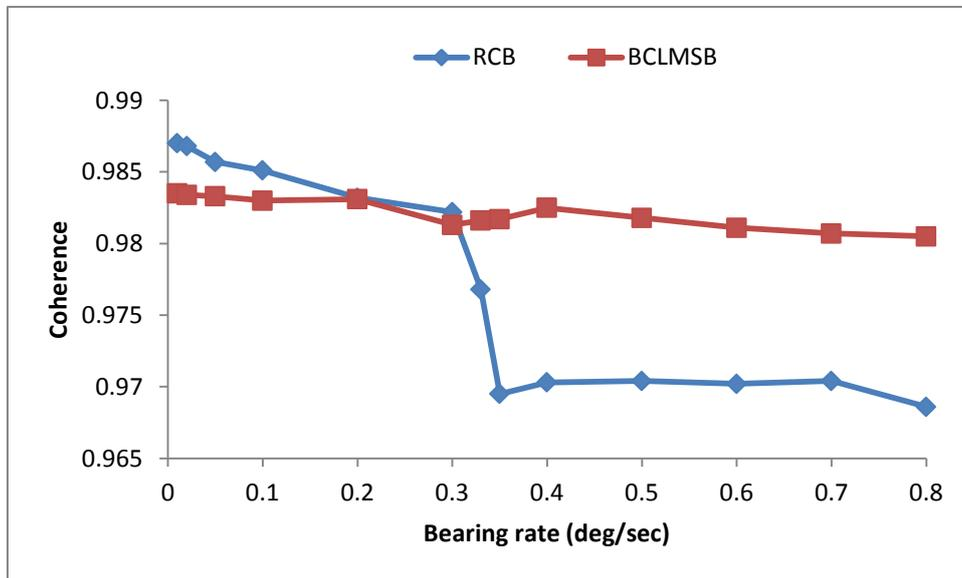
Figure 4. The effect of bearing rate of the moving signal source on the coherence achieved by RCB and BCLMSB.
