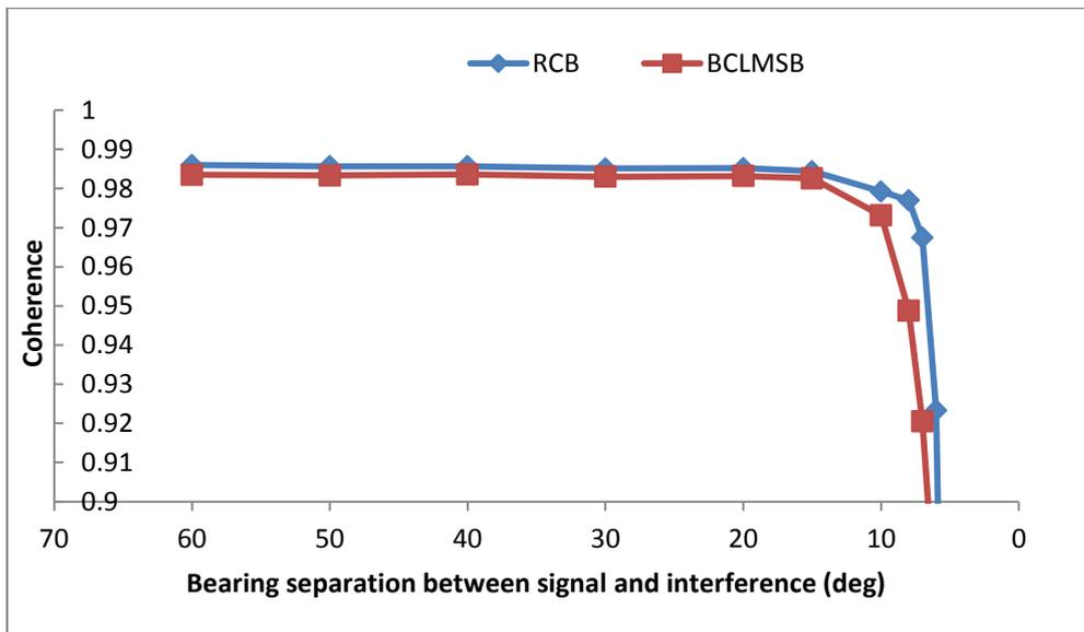
Figure 5. The effect of bearing separation on the coherence achieved by RCB and BCLMSB.
