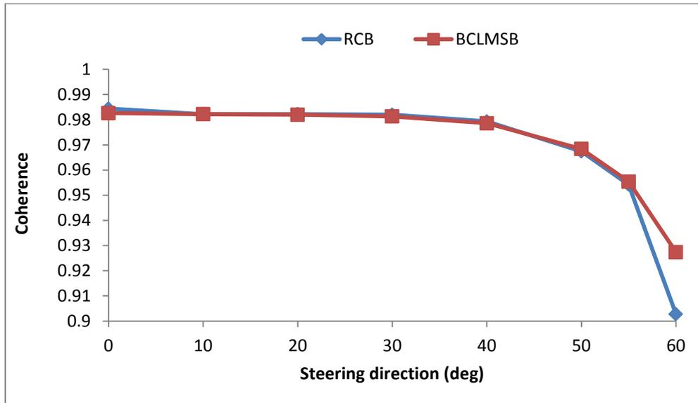
Figure 6. The effect of steering direction on the coherence achieved by RCB and BCLMSB.
