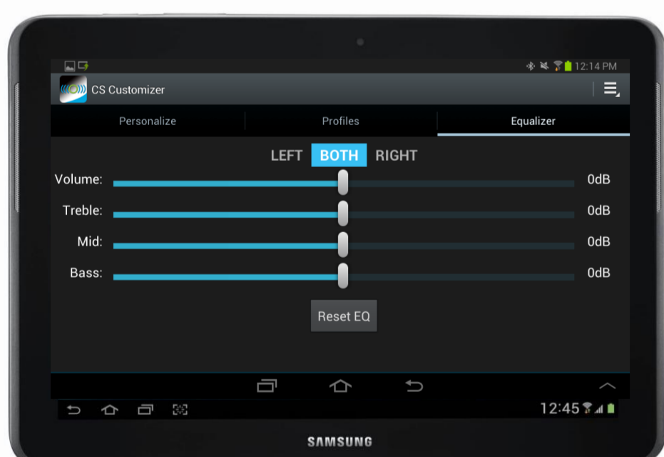
Figure 2. The fine-tuning screen of the self-fitting app, which allows users to adjust the overall gain as well as high-, mid-, and low-frequency gain.
