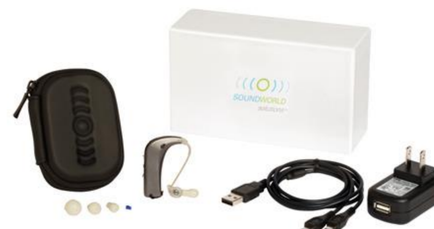
Figure 1. The rechargeable test device used in the study, which includes three ear tip sizes and adjustable tubing.
