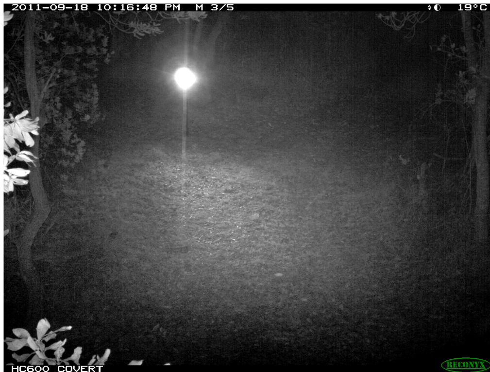
Figure 13. Infra red illumination of two opposing Reconyx HC600 camera traps simultaneously triggering. doi:10.1371/journal.pone.0110832.g013
