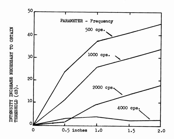
HORIZONTAL DISPLACEMENT OF EARPHONE FROM ITS POSITION WHEN ON EAR.
